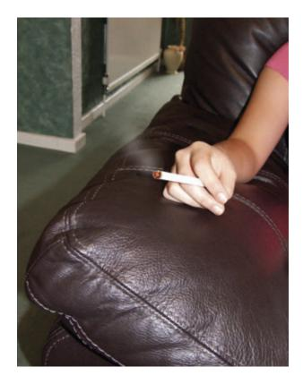
'Worst case' means the use of a filling that is likely to render the material combination most prone to ignition from a cigarette. Simply, a fabric can be tested over a filling that is either worse than any that is used or is the worst that can be used by an individual manufacturer. A positive test result indicates, but not necessarily confirms, that a particular fabric would be acceptable with other filling combinations.
